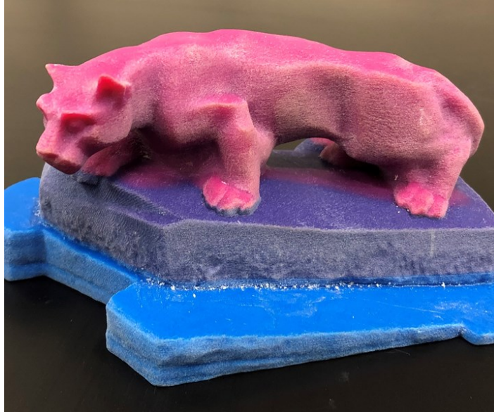
Illustration: sample object printed with MJ technique, which underlines the multi-color ability
